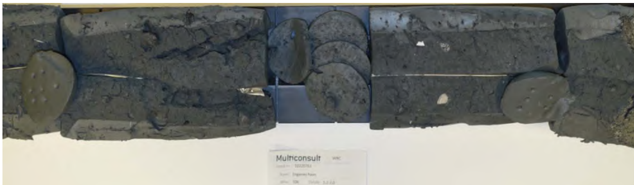
Figur 4-2: BP.106, 1,2-2,0 m – siltig, sandig leire.
