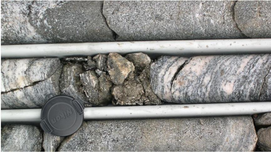
FIGURE 29: DRILLING CORE AT 33,5 M DEPTH AT THE MIDDLE BOREHOLE AT ÅKNES, SHOWING A CRUSHED AND BRECCIATED ZONE WITH SILT AND CLAY, REPRESENTING THE UPPER SLIDING ZONE. THIS SLIDING PLANE IS ALSO DOCUMENTED BY DISPLACEMENT IN DMS™ COLUMN (FIGURE 23).
