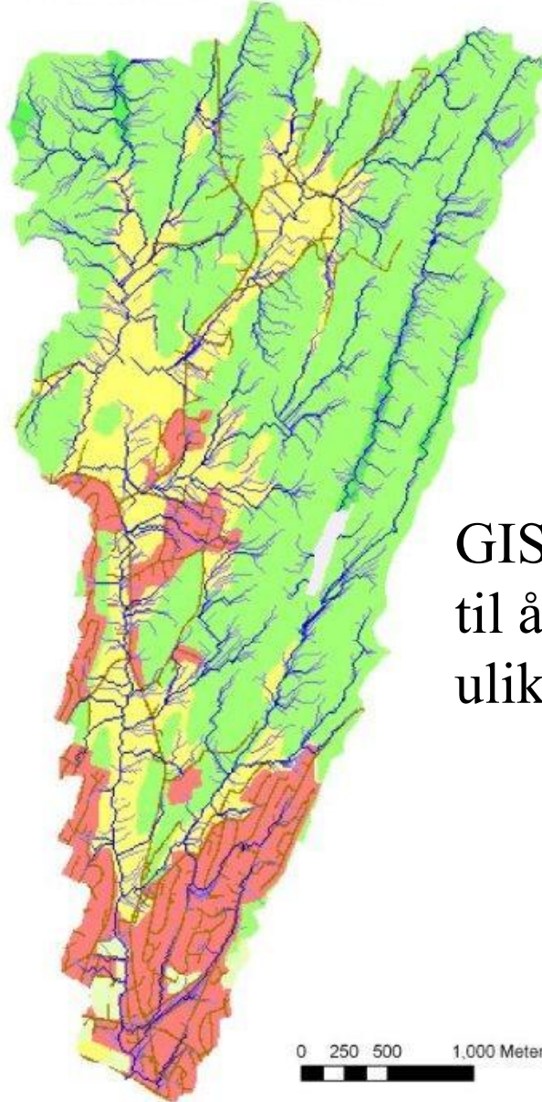
Surface runoff in the Fredrikstad-catchment for a 40 mm/2h rain storm
