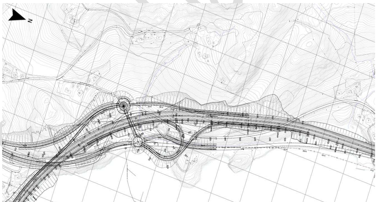
Figure 4-9: Drawing that shows the ramp design for alternative DR 2/3 north of Skulhusodden
