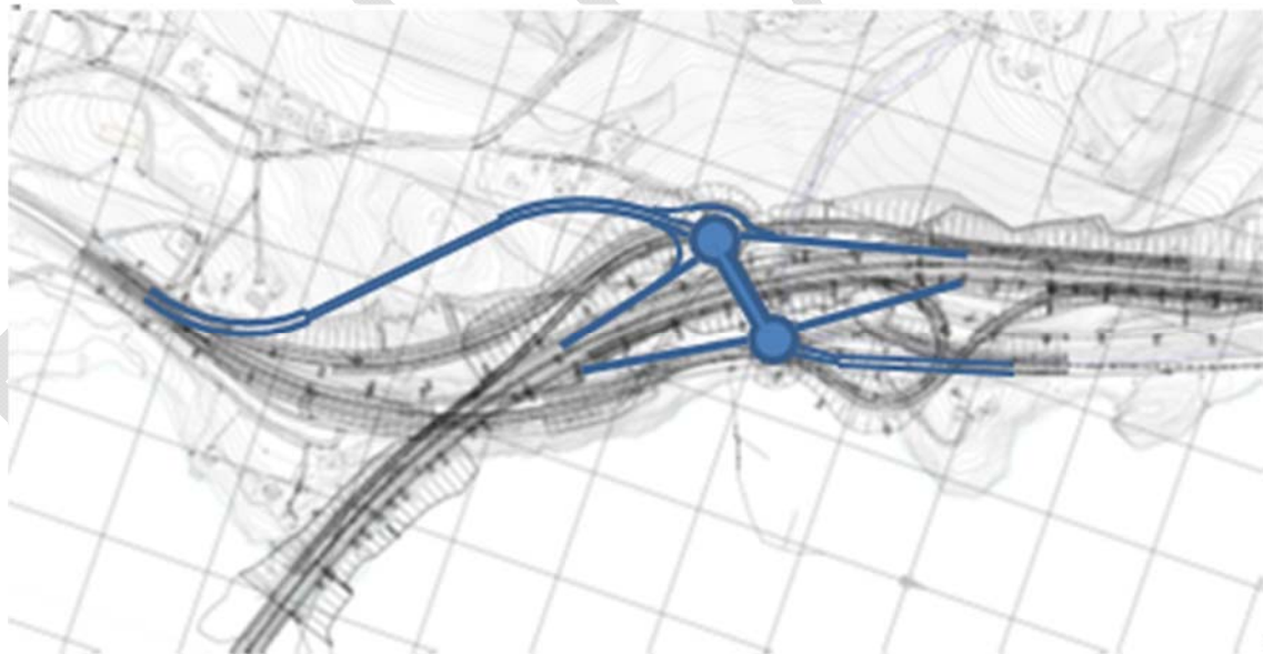
Figure 4-25: Suggested optimized alternative. DR 2/3. Local road, rv. 4, on- and off-ramps and “dogbone”-shaped ramp terminal are in blue. Illustration from Trafitec.
