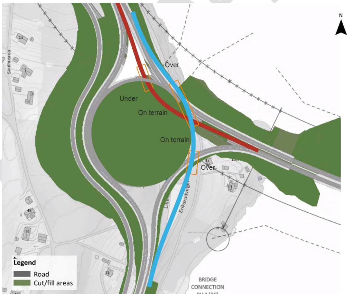
Figure 4-23: Roundabout with “flyovers” if needed when rv. 4 is expanded to a four-lane road
