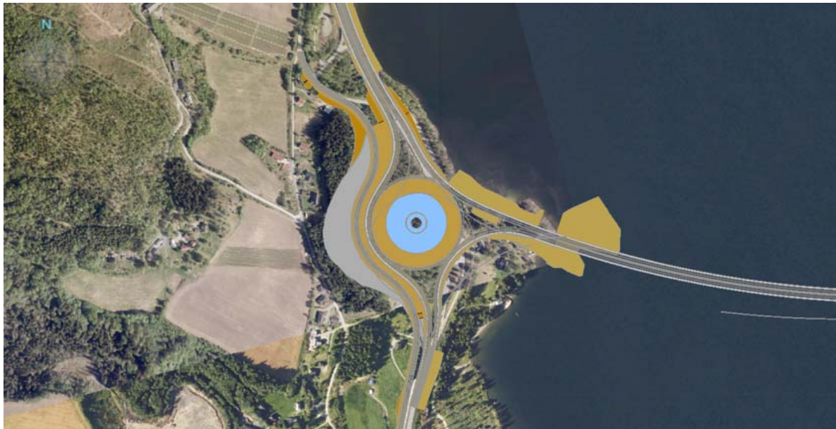
Figure 4-22: Overview of roundabout with curved bridge (RK 3AN) in the Skulhusodden area, shown on photo background
