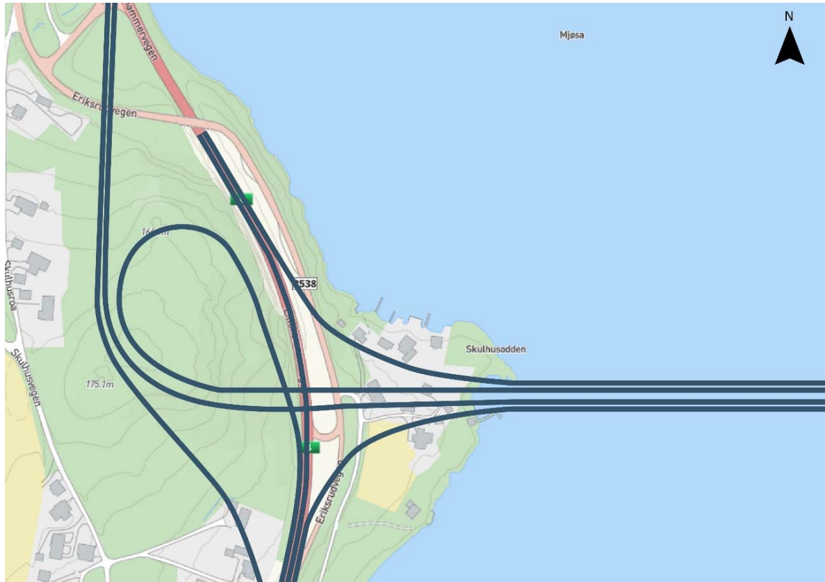
Figure 4-28: An illustration of an alternative to direct ramps with split lanes and reduced speed
