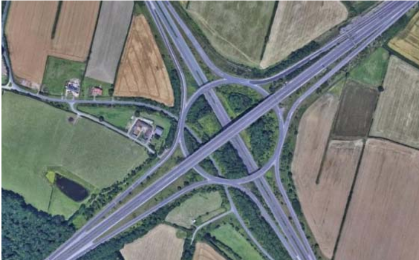
Figure 4-16: Example "flyovers" in a roundabout solution
