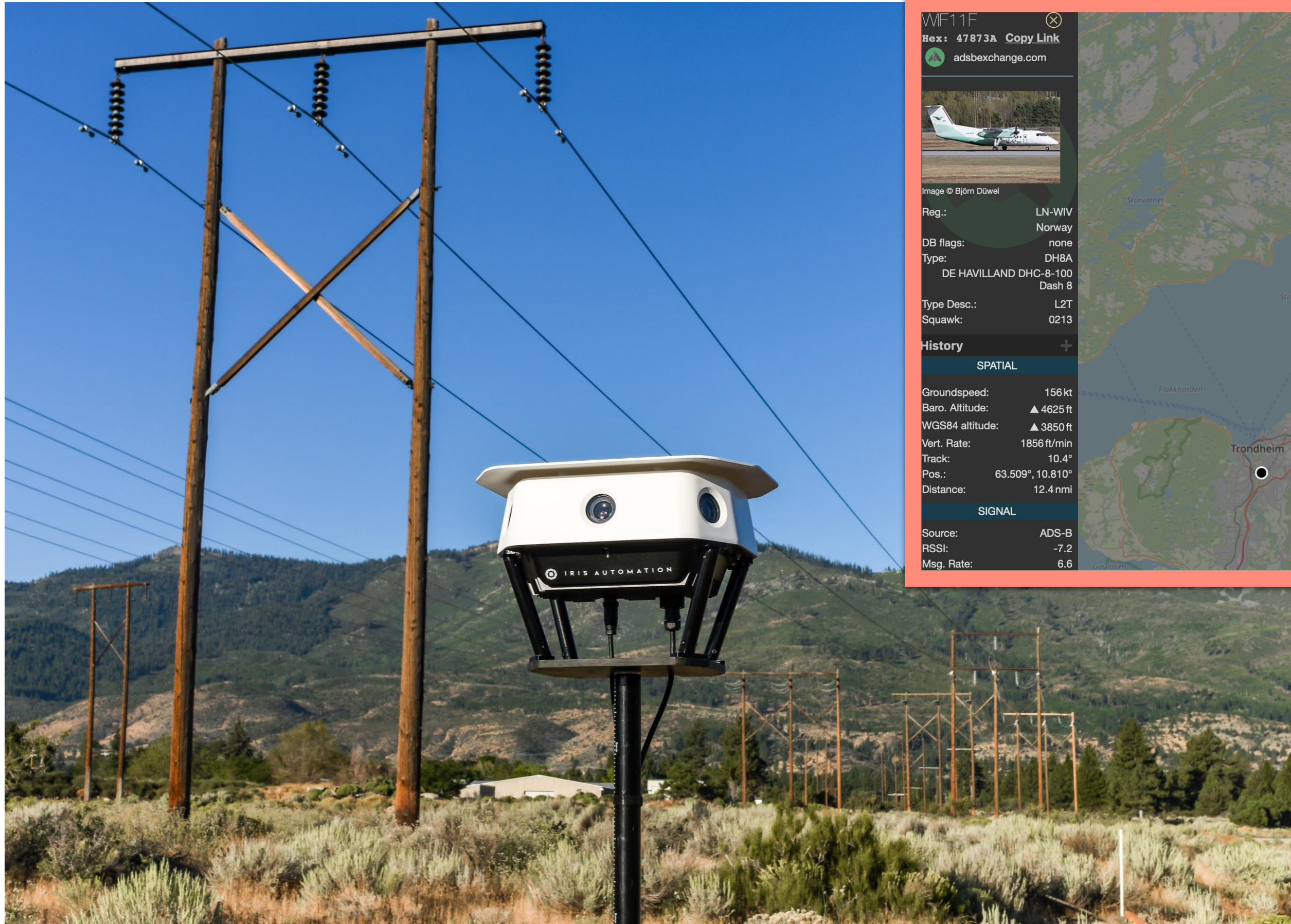
Automatic Dependent Surveillance–Broadcast (ADS–B) is an advanced surveillance technology that combines an aircraft’s positioning source, aircraft avionics, and a ground infrastructure to create an accurate surveillance interface between aircraft and ATC.
